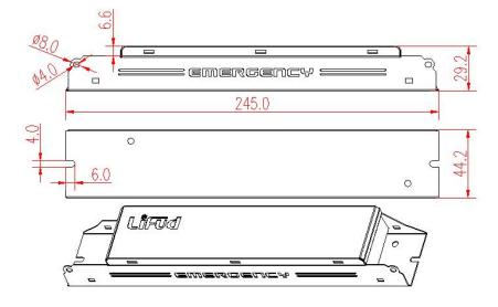
4.2 Dimension of the battery housing L\*W\*H = 279\*46\*25 mm
