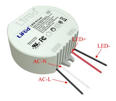
**Input wire:** UL1015 No.18 multi-stand wire, Black AC-L and White AC-N ,total length of 300mm ± 10mm, exposed 250mm ± 10mm, tail stripping dip tin 10mm ± 2mm
